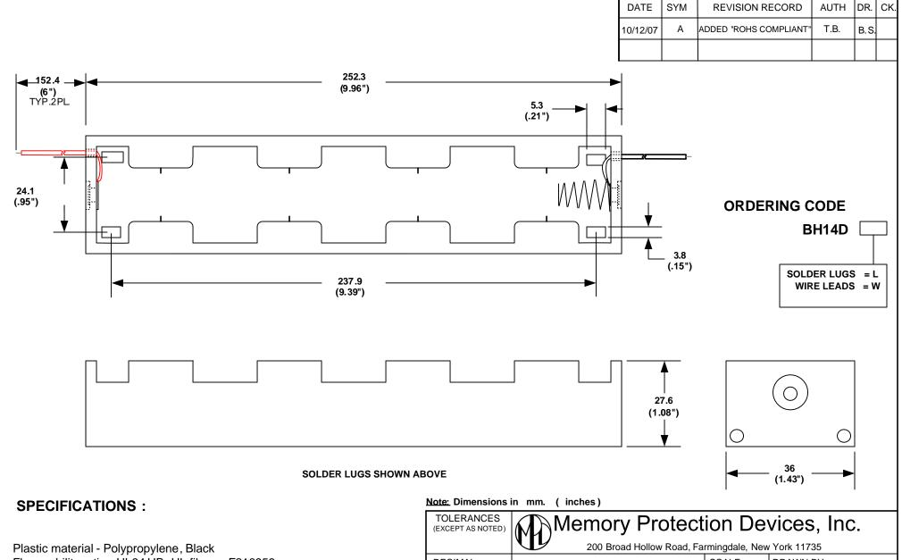
Flammability rating-UL94 HB, UL file no. E216959 Temperature Range: -10°C to +100°C Springs - nickel plated spring steel Rivets - Brass, nickel plated 9 Volts Snaps - Brass, nickel plated Contact resistance: Under  $50\text{m}\Omega$  for +/- contacts per EIA-540J000 ROHS COMPLIANT
